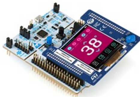
Figure 1. X-CUBE-DISPLAY running on NUCLEO-G071RB equipped with X-NUCLEO-GFX01M1
